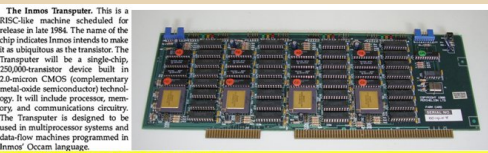
INMOS ANNOUNCES A 32-BIT 10-MIPS "TRANSPUTER" Inmos Corp. has announced the IMS T424 transputer, a 32-bit microprocessor with 4K bytes of on-chip high-speed (50-nanosecond) RAM. Inmos says the transputer will execute an average of 10 million instructions per second.
