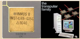
INMOS ANNOUNCES A 32-BIT 10-MIPS "TRANSPUTER" Inmos Corp. has announced the IMS T424 transputer, a 32-bit microprocessor with 4K bytes of on-chip high-speed (50-nanosecond) RAM. Inmos says the transputer will execute an average of 10 million instructions per second.
