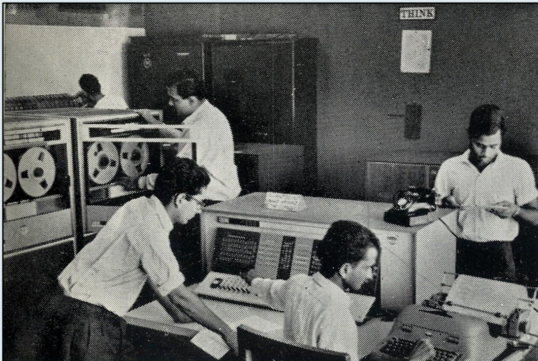
The IBM 1620 at IIT/Kanpur. R.N. Basu is mounting a tape. IBM Engineer Hinduja is standing in front of the console. M.N. Misra is operating the console typewriter. Source: IIT Kanpur 1965 Convocation Publication, IITK and CMU Archives
